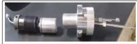
Limestone core samples and adjustable end plugs to fit core samples
