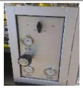
Front panel for maintaining in-situ reservoir conditions
